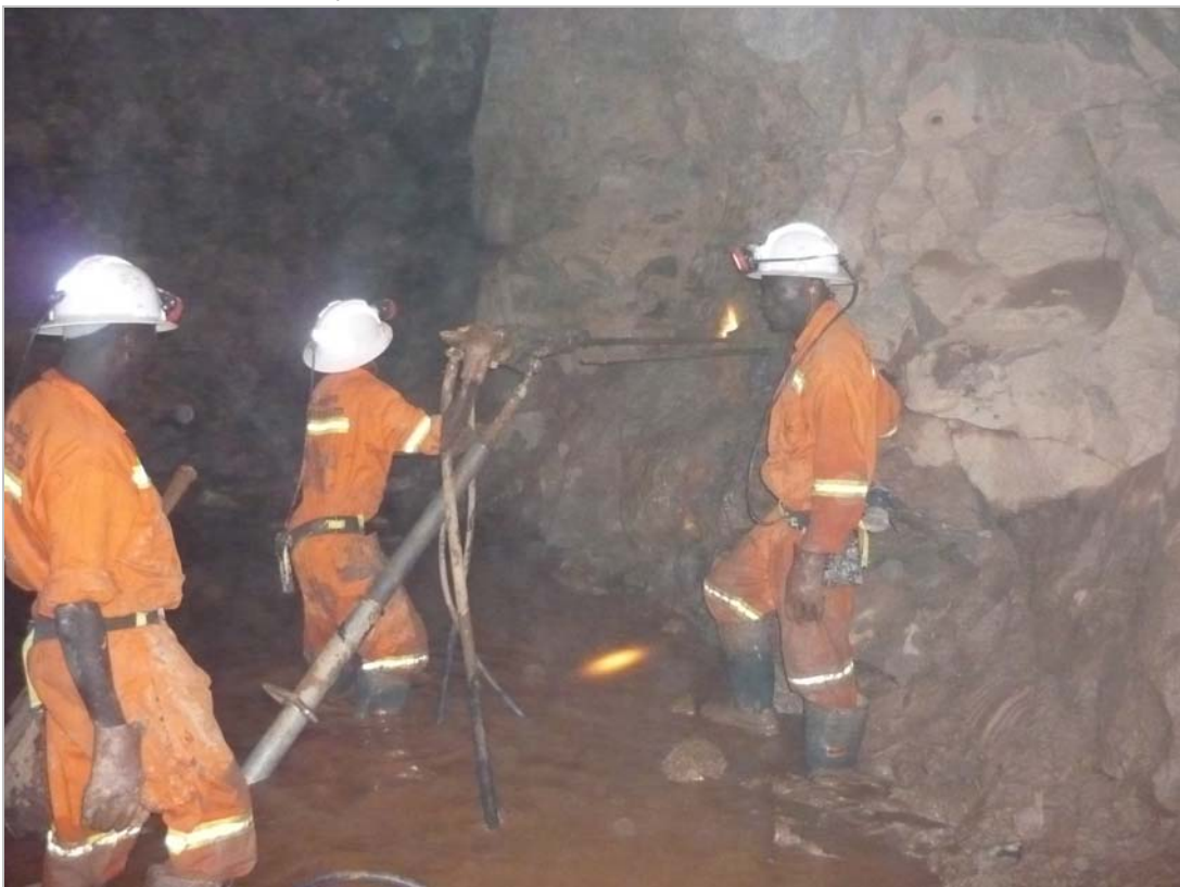
FIGURE 2 - Photograph showing underground miners at Perkoa drilling the working face for blasting.
